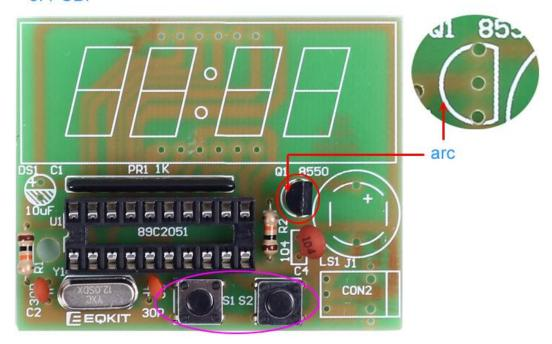
Step 5: Install 1pcs Power Socket at J1. 1pcs 10uF 25V Electrolytic Capacitor at C1 and pay attention to its installation direction.
